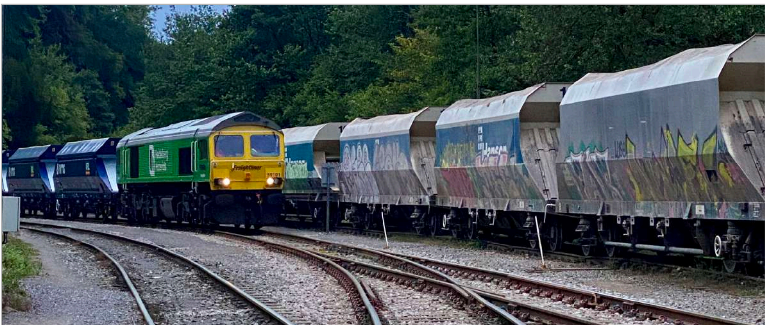
The new HOA hopper wagons pictured arriving at Merehead, replace an aging fleet of LTF and O&K JHA hopper wagons which were in service for 35 years. The new wagons are specifically designed to maximise payload efficiency and improve network performance by reducing travel times.
