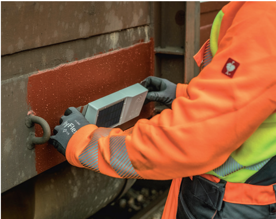
Every VTG wagon is to be fitted with a telematics system.
