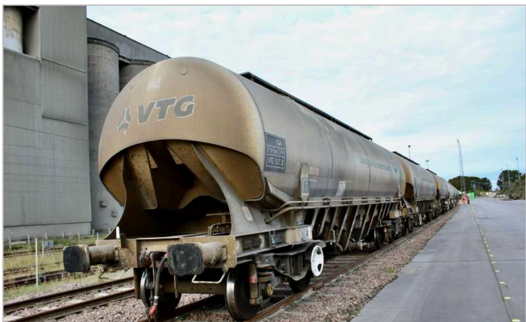
The JGA-M wagons play a vital role in the transportation of powdered cement from Tarmac's Dunbar cement plant in Scotland and their Tunstead Quarry in Buxton.
