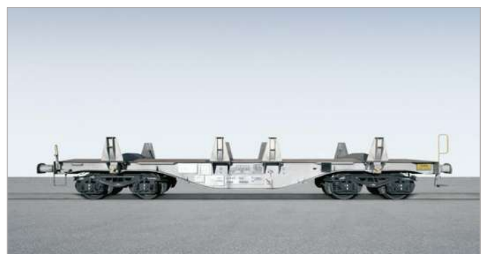
The VTG type F44.120E flat wagon offers optimal solution for the transport of hot steel slabs of different lengths and widths which can be loaded by a crane with grabs or magnets. Special load securing bolster beams on the wagons secure the load against sliding in lateral and longitudinal direction.
