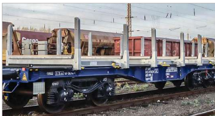
The Sggrs 2 x 40' + VTG Modupallet with its volume optimised construction allows more product to be loaded on to each wagon. The ModuPallet Steel is a perfect match and VTG's modular solution for the transport of steel products such as slabs, blooms, tubes and rails.
