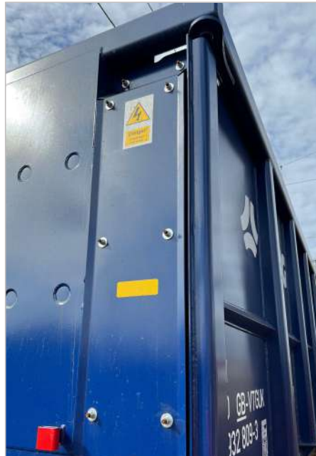
The latest JNA-T box wagons have been fitted with 'step prevention panels'.
