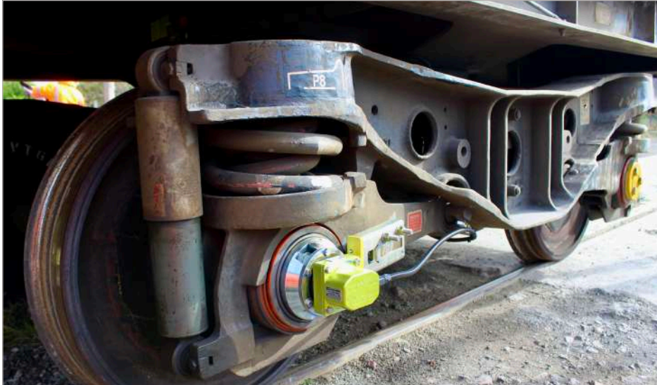
Each of the wagons has been fitted with new wheelsets containing four axle end generators which provide power to the Wheel Flat Prevention system.
