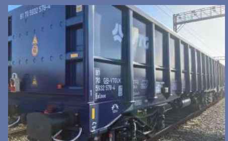
VTG's new JNA(T) box wagons include a high impact floor to reduce the risk of damage.
