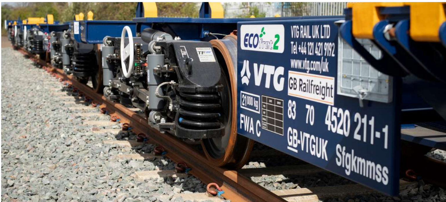
VTG's revolutionary Ecofret2 platforms are fitted with a bogie design incorporating rubber suspension components and hydraulic damping.
